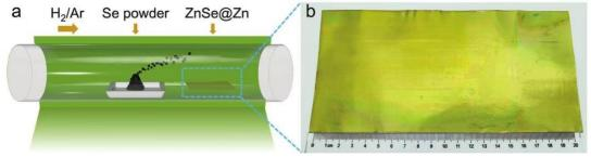
Figure 2: Schematic diagram and macrograph of CVD growth of a uniform ZnSe layer on zinc foil [9]
